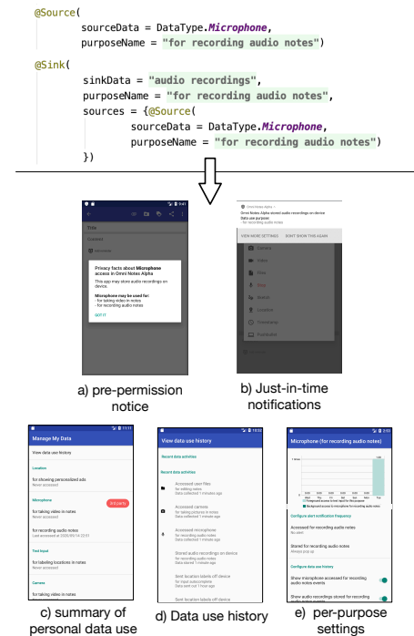
Developers add privacy annotations , and Honeysuckle converts them to a variety of of in-app privacy notices
